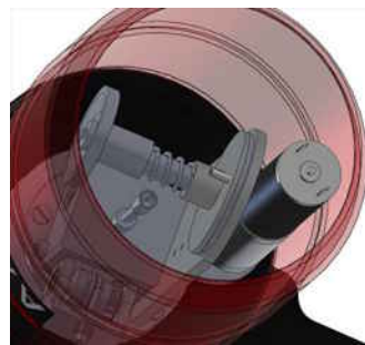
Wire supply rotates along with head
